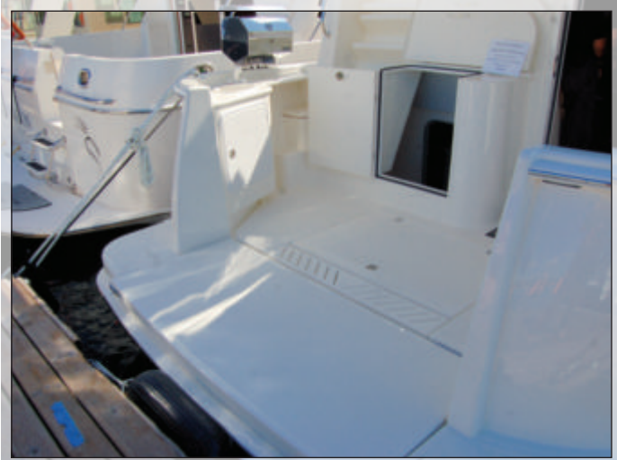
This shot of the cockpit shows the transom tailgate lowered and the engine room access open at the aft bulkhead.
